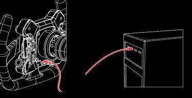
If there's no response when using the auto pairing mode, attach the included USB Type-C cable from the socket at the back of the wheel to the socket on the PC to manually sync the frequency (Please unplug the cable before driving in wireless mode)
