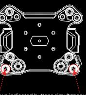
Press and hold the two indicated buttons simultaneously for 5 seconds to reset the wheel back to factory default settings.
