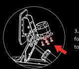
3.2 Attach the P-HPR GT using four M4-6 Pan Head Screws to complete the installation.
